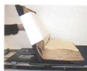
A book cradle that is used with a copy stand for taking digital images
